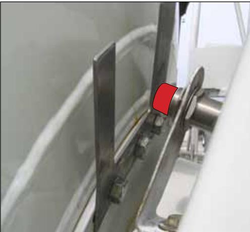
Sensor is mounted perpendicular to fork-plate (red cap face first).
